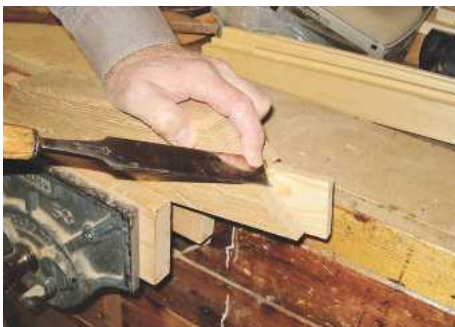
▲ Pic.16 ...when cutting the ovolo profile on the window rails
